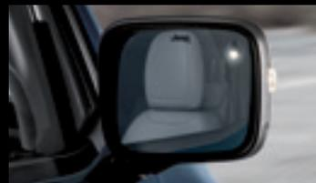
**TOTWINKEL-ASSISTENT UND QUERBEWEGUNGSERKENNUNG (Blind Spot Monitoring and Rear Cross Path Detection)**
